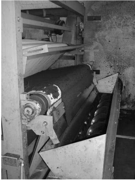
Figure 2: Belt Press Separator Outlet and Press “Cake”
