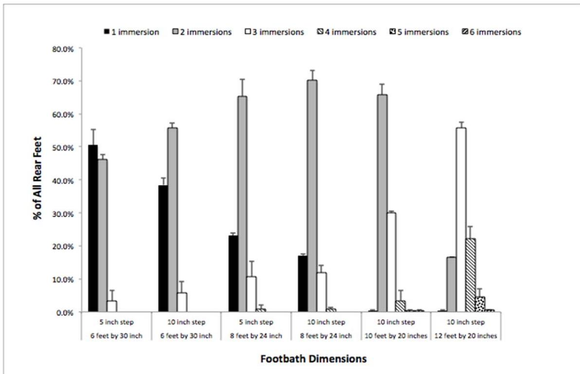
We advocate footbath designs that are 10-12 feet in length with a 10 inch high step-in, as narrow as 24 inches, with sloped enclosed side walls (Figure 5). When filled to 4 inches in depth, this bath still maintains a final bath volume of around 50 gallons. We do not recommend the use of wash baths.
